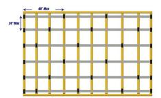
The Staggered Method is the most effective way to install MetroFlex MF-RIC clips, but uses more clips than the Stack Method. The same 48" max rule applies, but clips on the adjacent hat channel are not placed on the same stud as above or below. Simply move the clip one stud to the left of the clip above. Clips must be installed on both ends of the wall to ensure adequate support.
