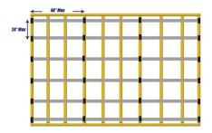
The Stack Method is the easiest way to install MetroFlex MF-RIC clips. Clips are stacked no more than 48" apart horizontally on the studs and the same stud location is used for all hat channel. Clips must be installed on both ends of the wall to ensure adequate support.
