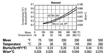
$<sup>^{*}</sup>$  Apparent thermal conductivity values are determined by applying procedures dictated per ASTM C1045 on test data obtained using ASTM Test Method C335. All values are based on nominal manufacturing and testing parameters, are subject to normal variation, and are not guaranteed for specification purposes or otherwise
