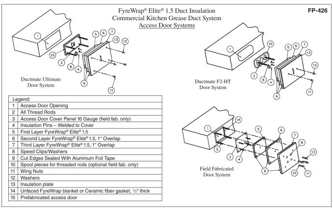
Figure 3. Firestop Installation
