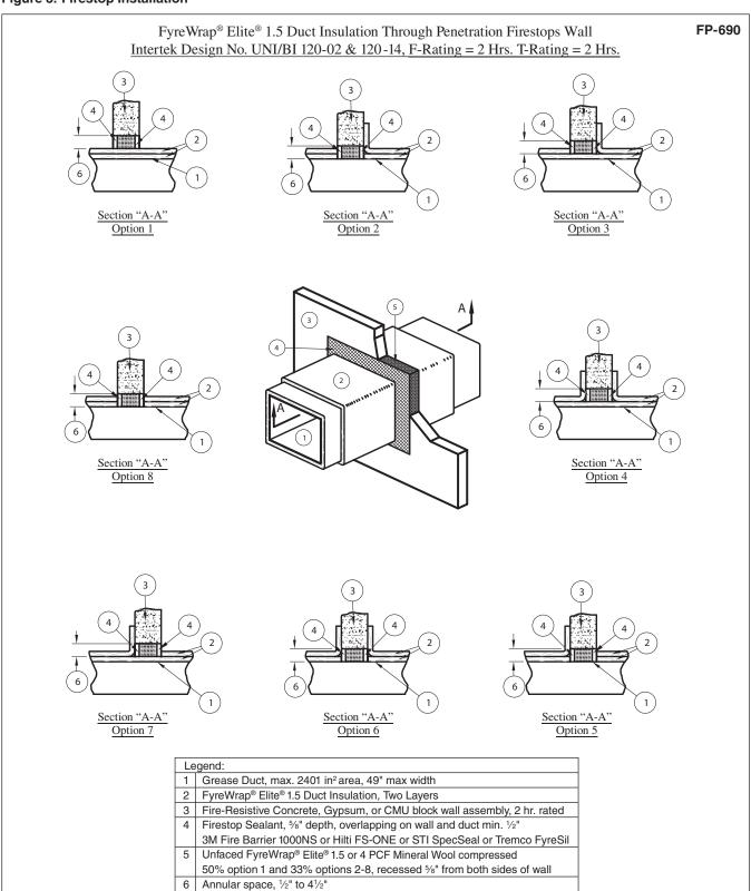
Figure 4. Firestop Installation
